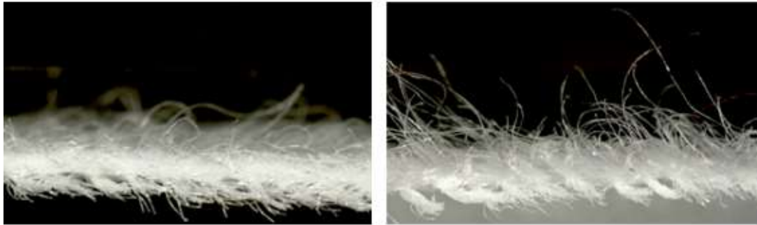
Figure 6. Images on the surfaces of PET and PET/PLA fabrics after 1000 cycles abrasion at natural state
