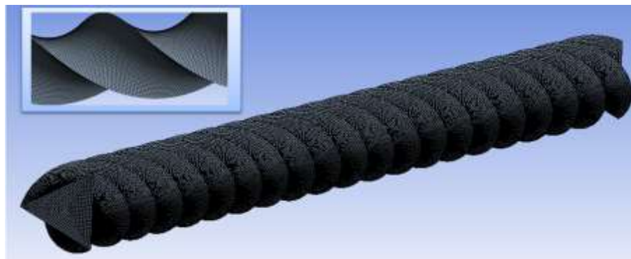
Fig. 2. Generated tetrahedral mesh for a twisted tube at Tr = 5
